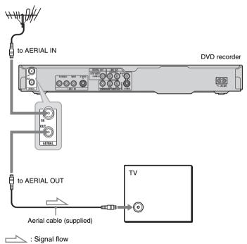
**1** Disconnect the aerial cable from your TV, and connect it to AERIAL IN on the rear panel of the recorder.
